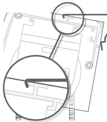
Holding the rail at an angle, situate the T-shaped lip on the top of the cassette into the front lip of the bracket.
