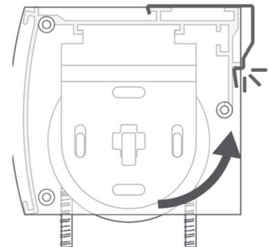
Twist the back of the cassette upwards until it snaps into place against the back lip of the bracket.
