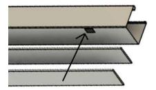
The battery is shipped partially charged. We highly recommend to fully recharge it for about 4-6 hrs before installing the blind in the brackets. Connect charger from the power supply to the Battery charging port, located in the **right hand side**, below the head rail as shown.
