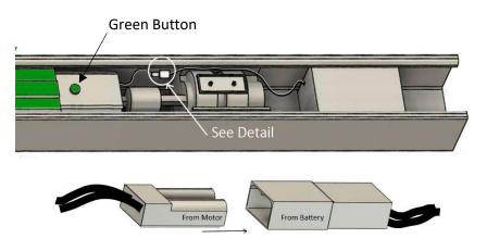
You should get a small motion from motor indicating the battery connection was successful.
