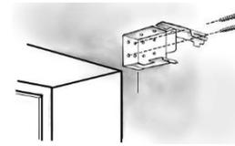
Measure the headrail length and mark with a pencil on the wall the position where the ends of the headrail will be located. Be sure these marks are centered on the window and use the level to determine the vertical position. Now, mark the position of the End Brackets, ¼" outside of the headrail marks. These will be the outside position of the End Brackets. Attach the brackets against the wall with the screws provided.
