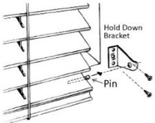
Insert the Pin in the pre-drilled hole in the Bottom Rail and with the Pin in place, locate the position on the wall of the Bracket. Mark the location of the screws and drill.
