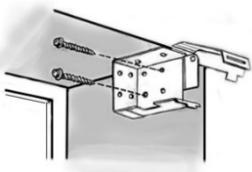
Open the bracket by applying pressure on the latch. Brackets are marked LH (Left Hand) and RH (Right Hand). Screw into the window frame through the holes on the inside of the bracket as shown. Always use at least two screws per bracket. Screws mounted horizontally will have more strength.
