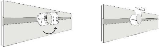
Insert each Magnetic Valance Clip in the slot behind the wood valance and spread them evenly along the valance slot. Turn the Valance Clips Up. Hang the Valance from the top of Headrail.
