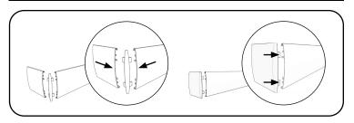
**Metal returns** (Outside mount only) include a plastic corner connector. **Plastic returns** (Inside mount with Outside Mounted fascia) snap on the end of the fascia.
