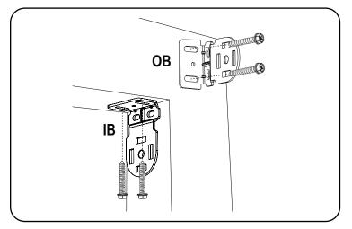
Secure the roller shade installation brackets with the supplied screws. If shade was ordered as outside mount (OB), attach the supplied screw covers on to the bracket for a finished look.
