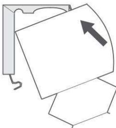
Situate the front lip of the headrail into the front hook of the bracket.
