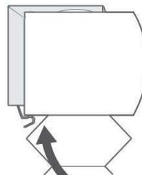
Push the back of the headrail upwards to engage the metal clip at the back of the bracket.
