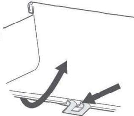
To remove the blind from the brackets, insert a flat head screwdriver into the tab protruding from the bottom of the rail, then gently pry it back while tilting the back of the rail downwards. Repeat this carefully for each bracket to release the rail.
