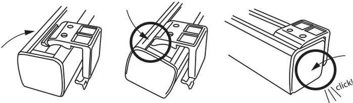
tab at the bottom of each bracket snaps onto the back of the head rail. Check carefully to assure that each bracket is properly secured.
