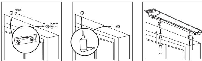
One bracket should be positioned about 2" to 6" from each end of the headrail.
