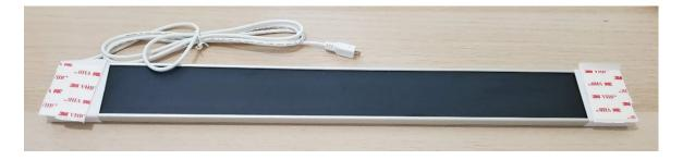
Remove the "face" of the applied adhesive. Position the solar panel facing to outdoors, then press entire panel with firm, even pressure into the glass for 10–15 seconds. The panel is now supported by the adhesive to glass bond but will require 24 hours of cure time to allow full strength characteristics. Do not disturb during this period.
